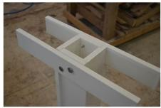
Step #3: Attach Table Top horizontal support bars and fasten with provided Stainless Steel screws in pre-drilled holes.
