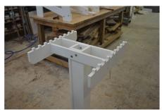
Step #4: Insert Dog Bones into slots - be certain to put the wider end pieces into the outside end slots. Attach using the provided Stainless Steel fasteners in the pre-drilled holes.
