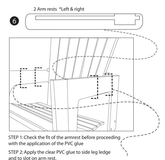
STEP 3: Clamp 2 parts together (or wrap firmley with heavy tape, or place heavy flat object on top) to assure a tight bond.
