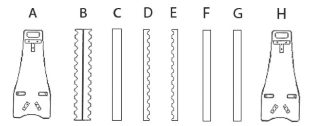
STEP 1 Insert item C into the bottom side of item B and insert screws into the pre-drilled holes. Note, item C is 3 1/8" wide and is the wider of the 3 support cross bars.
